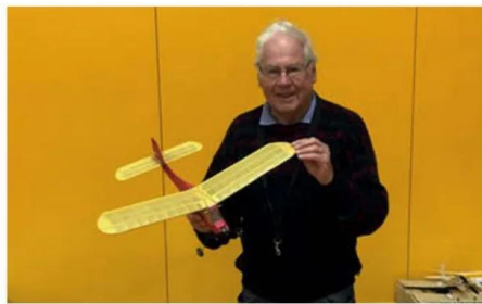
Ian Jemmeson's 60% size PAAGeboy for Indoor Flying, still flying well five years after it was built. It has a small 2s Lipo battery and Spectrum Rx on 2.4G driving a small brushless motor.
