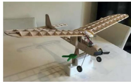
Ian Jemmeson's PAAGeboy for Indoor flying, C of G being checked before covering the model.
